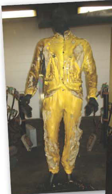
Brand-X rainwear commonly labeled as flame resistant (FR), however demonstrated significant melting, dripping, shrinkage, break open, and ignition in a flash fire test.
