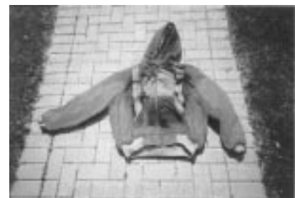
3. Non-flame resistant wool jacket , with flame-resistant cotton shell (Millworks Manufacturing) survived a 30 kA/10 cycles arc 12 in. away. Both inside and outside of jacket were exposed
