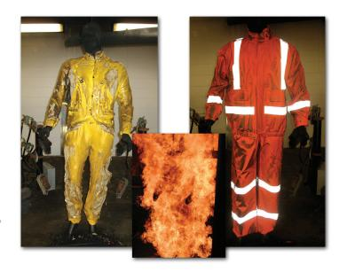
In the utility industry, ASTM F1891 is the rainwear performance standard for electric arc flash. For gas utilities and combination utilities, ASTM F2733 is the rainwear performance standard for flash fires. Therefore, if you are wearing daily wear garments that comply with ASTM F1506 or NFPA 2112, your rainwear must be compliant to F1891, F2733 or both.
